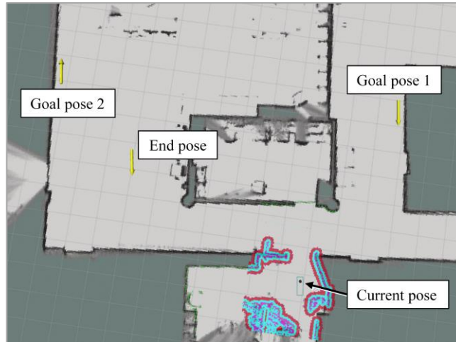
Fig. 3. Generated map of the environment with goal poses of the inspection mission.
