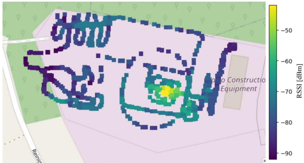
Figure 8: Results of the signal strength test displayed in the signal strength map overlay
