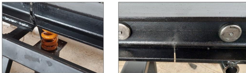
Figure 10. Translation spring substituting pinned support (left) and cut close to midspan (right).
