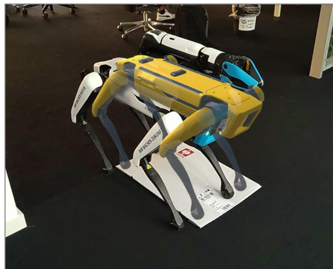
Figure 6. Alignment of the virtual and the real Spot at \{G1\} during mission recording.
